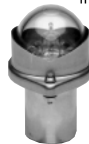
THE WHELEN A625 STROBE LIGHT HEAD ASSEMBLY is the same physical size as the Model S tail position light and will fit the same mounting adapter. It is used in enclosed-type wingtips. The unit fits nicely behind the position light on conical camber wingtips, see reference installation instructions on page 9 of this manual. Parts breakdown shown on Pg. 19, Fig. 25. SUPERSEDES A430.
