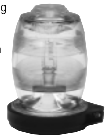
THE WHELEN A470A STROBE LIGHT HEAD ASSEMBLY is designed to produce light 360 degrees around the aircraft. The A470A incorporates a vibration proof strobe light flash tube which also allows flush mounting. The unit mounts on the aircraft using Whelen's H102 "B" or H103 "A" mounting adapter (see Page 5), see reference installation instructions on page 11 & 12 of this manual. Parts breakdown shown on Pg. 19, Fig. 27. SUPERSEDES A470.
