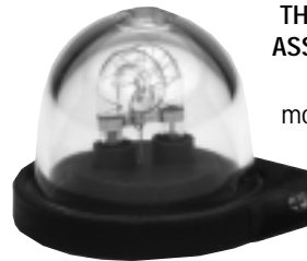
THE WHELEN A470A STROBE LIGHT HEAD ASSEMBLY is designed to produce light 360 degrees around the aircraft. The A470A incorporates a vibration proof strobe light flash tube which also allows flush mounting. The unit mounts on the aircraft using Whelen's H102 "B" or H103 "A" mounting adapter (see Page 5), see reference installation instructions on page 11 & 12 of this manual. Parts breakdown shown on Pg. 19, Fig. 27. SUPERSEDES A470.
