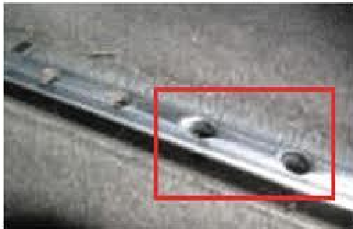
Worn seat track stop hole
